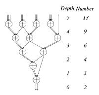
Fig. 3. Example of carry-save adder tree.
